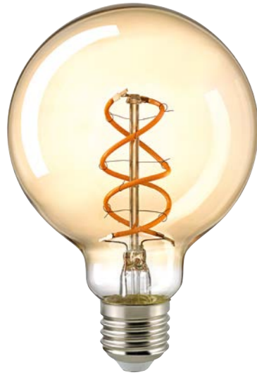
LM FILAMENT CURVED 6125801 leuchtmittel, glas, gold bulb, glass, gold H 14 cm x Ø 9,5 cm 4 Watt, LED, 1800K, 250lm, E27
